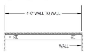
If GAMMALUX *EZ-TELE*<sup>™</sup> is not selected, the run or fixture is built to the exact dimension provided and will have no field adjustability. The exact fixture dimension must the signature approved (Verify In Field) to allow Release to Production.
