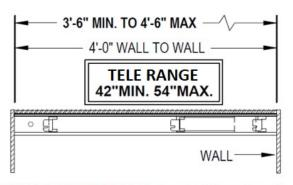
With GAMMALUX *EZ-TELE™*, the run or fixture has 6" of adjustability above and below the ordered (example 4') dimension. If the final dimension is within the fixture's adjustability, no field dimension is required.
