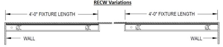
RECWL = only the left end of the fixture touches an adjacent wall. The other end will have the same ceiling trim as the front of the fixture. RECW**R** = only the right end of the fixture touches an adjacent wall. The other end will have the same ceiling trim as the front of the fixture.
