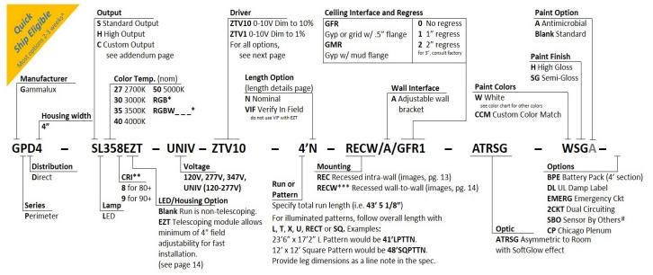
\*\* 90+ CRI increases watts nom. 14.5%. \*\*\* Field dims. required if not using GAMMALUX EZ-TELETM. # Sensor by Others (consult factory). \*Some restrictions apply. Check our Quick Ship Guide for details.
