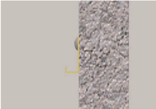
1) Adjustment Trim is added to the wall at a pre-determined height.
