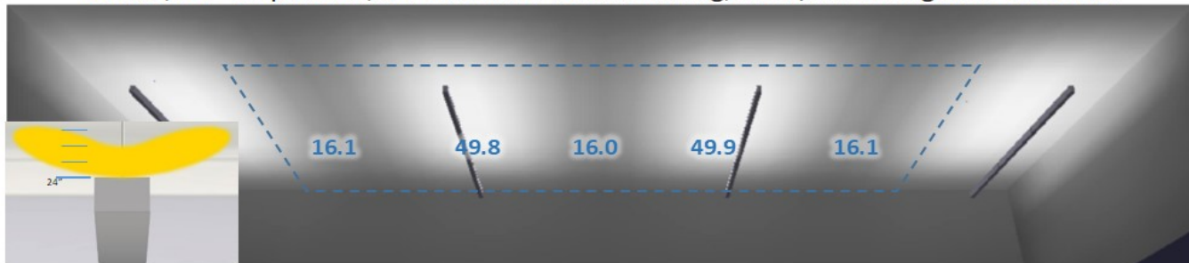
GGMS, 24" suspension, 14' on center row mounting, max\min ceiling ratio of 3.12:1
