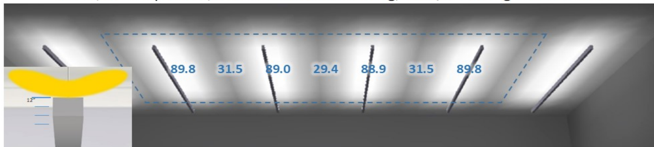
GGMS, 12" suspension, 8' on center row mounting, max\min ceiling ratio of 3.02:1
