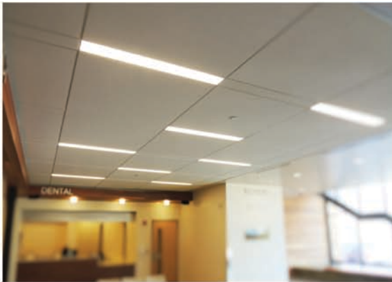
Flush with 15/16" grid (T1W)
